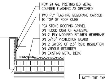
NOTE: THE EXISTING HVAC UNIT IS REQUIRED TO BE LIFTED TO ALLOW FOR THE APPLICATION OF TWO PLY FLASHING MEMBRANE ON TOP PRIOR TO INSTALLING THE METAL COUNTER FLASHING ON TOP, THEN LOWER THE HVAC UNIT ON TOP THE METAL COUNTER FLASHING
