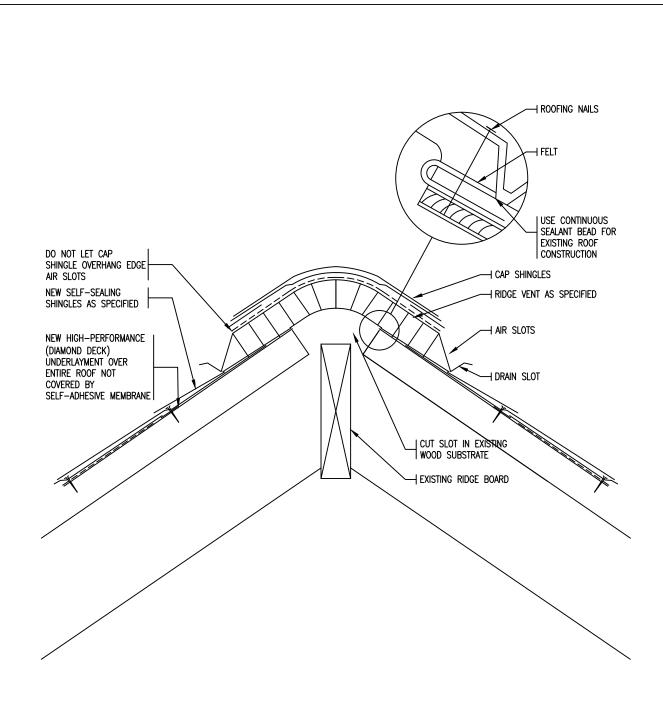
NOTE: WOOD CEDAR SHAKES ARE REQUIRED TO BE INSTALLED AT EACH END OF RIDGE VENT (COVERED WITH EAVE PROTECTION) FOR A GRADUAL CONTOUR OF SHINGLES OVER TOP
